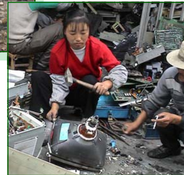
A worker in China smashing CRT monitor to remove copper. Dumped monitor glass later leaches lead into the groundwater.
